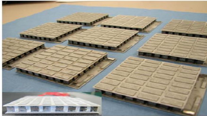
Figure 5.1 Skutterudite modules were fabricated by Marlow [36].
